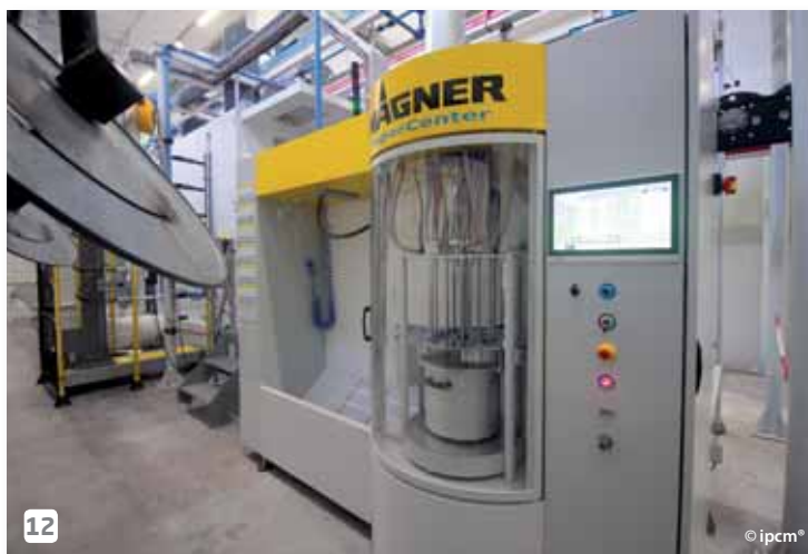
12 The brand new "SuperCenter" powder unit by Wagner Spa the powder coating system is equipped with.
