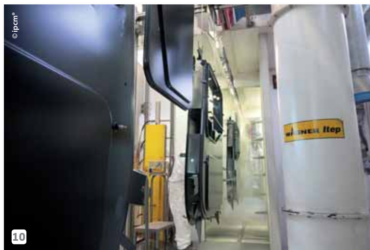
10 One of the many Wagner booths the powder coating systems are equipped with.
